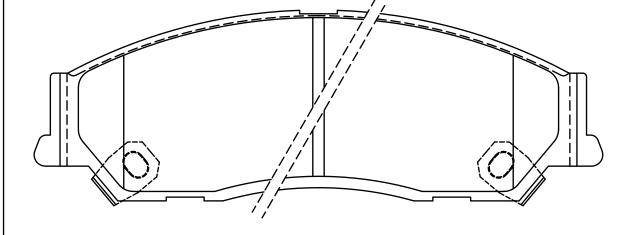
SET: 2 PIECES WITHOUT WEAR INDICATOR SPRING 1 PIECE WITH RIGHT WEAR INDICATOR SPRING 1 PIECE WITH LEFT WEAR INDICATOR SPRING
